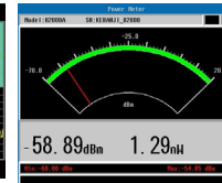
Agilent U2000 Series USB power sensor support (Option PWM)
